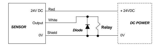
NOTE: Don't make any lines be electrically shorted with other lines when the power is applied. Damages may occur on the sensor.
