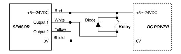
When one of the output lines is not used, it will be recommended to connect with 0V firmly for avoiding unexpected shortage with the red lead by an unconnected free lead end.
